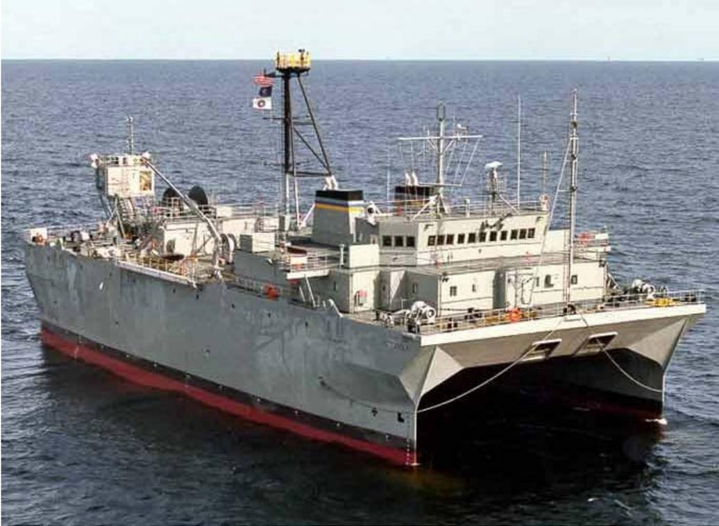
Figure 1-2. VICTORIOUS Class (T-AGOS 19 Class) Ocean Surveillance Ship.
